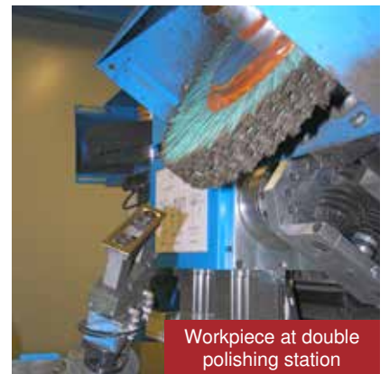
4 workpiece holders each with 2 axes, 1 grinding unit with 2 grinding stations, 2 double polishing units each with 2 polishing stations. All stations 5-axis
