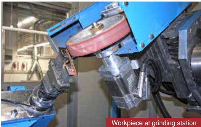
4 workpiece holders each with 2 axes, 1 grinding unit with 2 grinding stations, 2 double polishing units each with 2 polishing stations. All stations 5-axis
