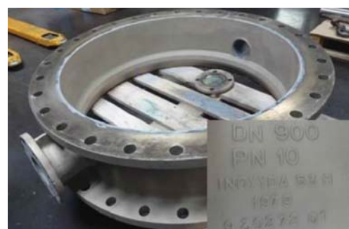
Aluminium bronze valve body during maintenance after 30 years (credit EDF).
