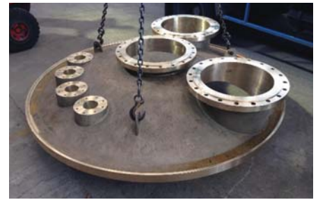
Weldless Inoxyda 3P Aluminium bronze casting.
