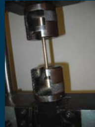
Test bar ready for tensile test.
