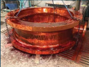
Dye penetrant test of pre-machined valve body (Credit Inoxyda).
