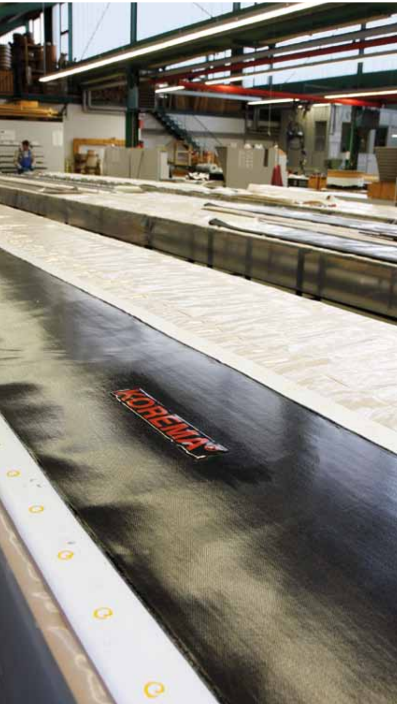
Production of belt type expansion joints
